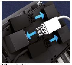
**3** | Connecting lines Select cables according to colour (black: general net, white: data processing net) and length. Insert the socket component of the 3-pole connecting line onto the snap-in piece in the device cup.
